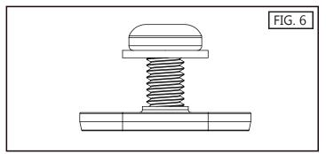
6. The sliding nut (Item #5) will go in the channel of the mpower traffic controller (See FIG. 7 and FIG. 8).
