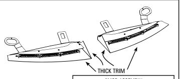
3MOD ASSEMBLY (COMPATIBLE WITH STANDARD OVERHEAD CONSOLE AND OPTIONAL FRONT READING/MAP LAMPS)
