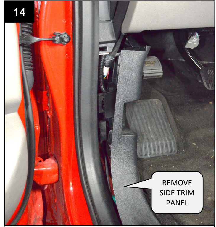
REMOVE SIDE TRIM PANEL LOCATED BY EMERGENCY-BRAKE.
