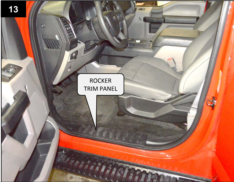
REMOVE ROCKER PANEL IN FRONT AND REAR DRIVER SIDE.
