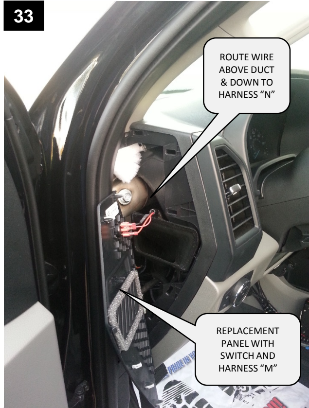
AFTER REMOVAL OF FACTORY TRIM PANEL, REPLACE WITH NEW TRIM PANEL WITH SWITCH. RUN HARNESS "M" DOWN AND PLUG INTO HARNESS "N" CONNECTOR.
