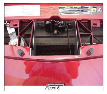
8. After latch and bracket are secured be replacing bolts, Place speaker at desired angle and tighten screws on both sides. (Ratchet with extension works best.)
