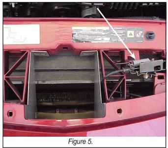
6. Lower speaker into place. Be sure that wire exits the bottom of speaker. Wire exit also functions as weep hole. Hand tighten screws into speaker by reaching where horn was located and was removed in step 4.
