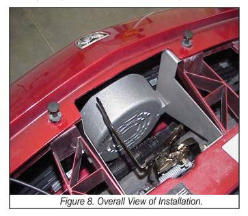
11. Close hood and check hood and body alignment. Adjust latch assembly if required for proper hood alignment.
