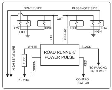
WIRING SCHEMATIC - 4 LAMP INSTALLATION
