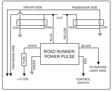
WIRING SCHEMATIC - 2 LAMP INSTALLATION
