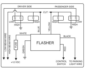
Wiring Schematic - 4 Lamp Install
