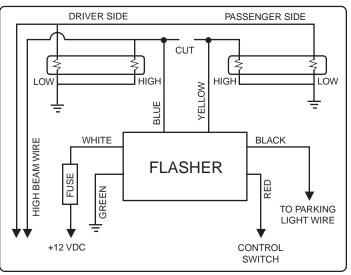
Wiring Schematic - 2 Lamp Install
