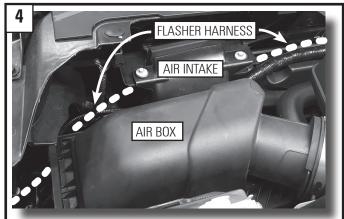
After bolting the flasher, run the long harness next to the air box and under the air intake, as shown above.
