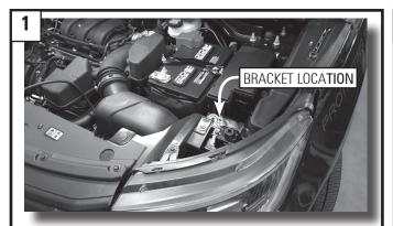
Driver side engine compartment shown. For ease of installation, remove both driver and passenger side headlights following the recommended manufacturers method.
