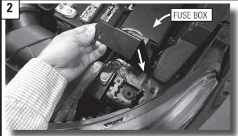
Slide the flasher bracket assembly between the fuse box and the grille reinforcement bracket, as shown above.
