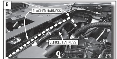
Continue routing the long flasher harness to the passenger side headlight assembly, as shown above. Plug flasher connector ends to each side of the headlight assemblies.
