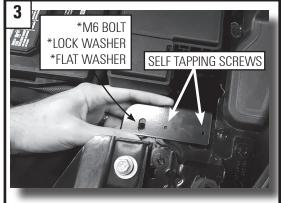
Using the supplied hardware included in the kit. Bolt the bracket as shown above.
