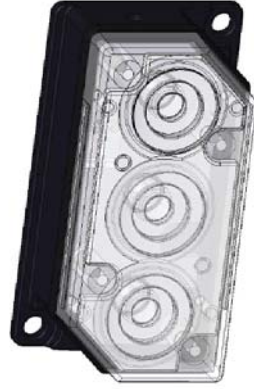
Drill Template for Mounting Holes/Cord Entry Template Shown Actual Size
