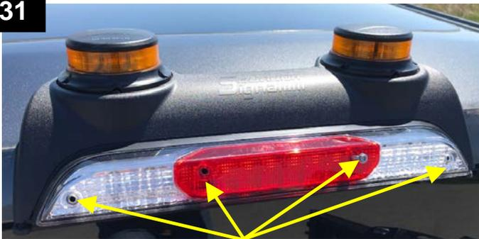
GARANTICE UN ALINEAMIENTO UNIFORME, SUJETE A MANO COMPRIMIENDO LA ESPUMA PARA **EVITAR FUGAS DE AGUA** E INSERTE LOS TORNILLOS 'A' Y APRIETE A  $2,0 \pm 0,3$  NM CON LLAVE Torx T-20 O VASO DE 7 mm
