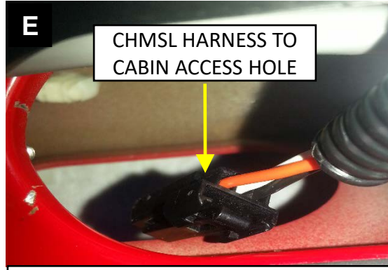
E CHMSL HARNESS TO CABIN ACCESS HOLE LED CHMSL – PREVENT LIGHT FLASH BACK INTO CABIN BY TAPING OVER ACCESS HOLE.
