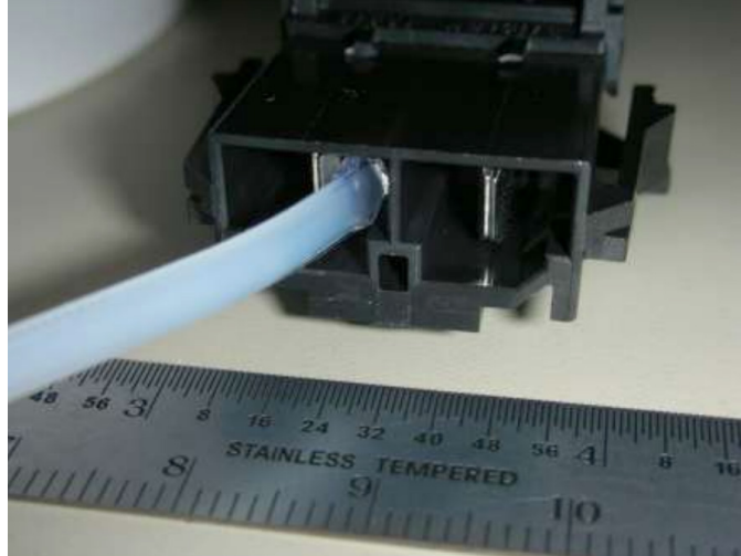
Apply Nyogel 760G to both sides of every male terminal.
