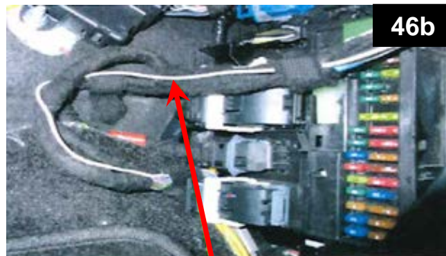
Run-start secured to BCM J1 harness
