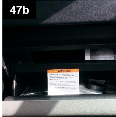
INSTALL WARNING CARD, 'K', IN GLOVE BOX
