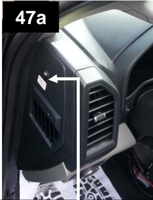
INSTALL SIDE PANEL LABEL 'E1' (IF DESIRED)
