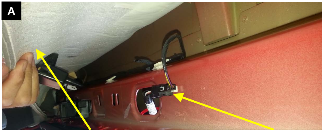
A PULL BACK HEADLINER TO EXPOSE CHMSL CONNECTOR
